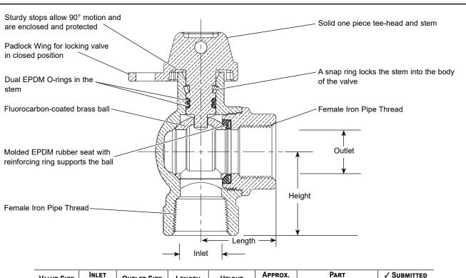
FEMALE IRON PIPE THREAD INLET AND OUTLET
