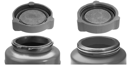
OLD STYLE CAPS Three-lug, 1/3-turn design rated to 200 psi (13.8 bar).
