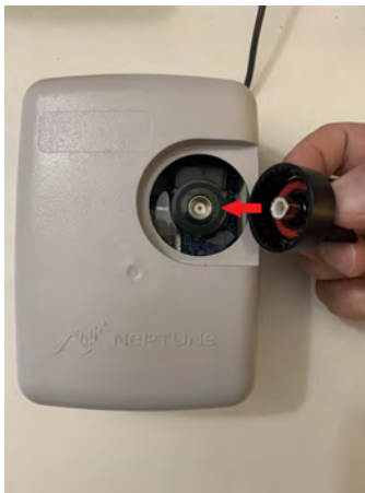
Figure 56 – Cellular Endpoint Conductor Pin
