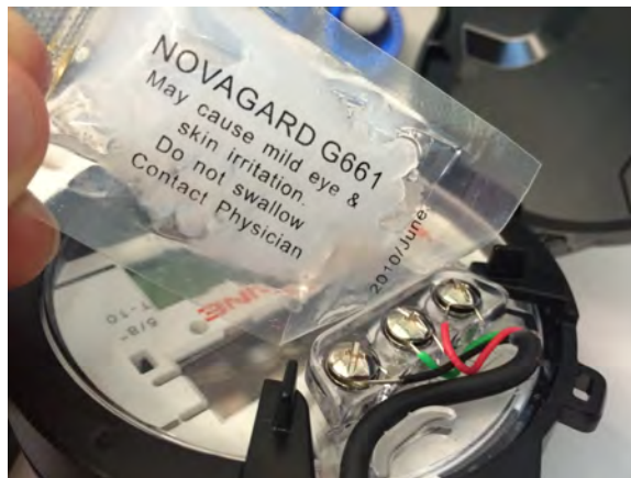
Figure 10 – Application of the Sealant
