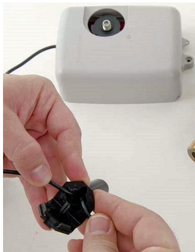
Figure 16 – Gray Wires in Slot
