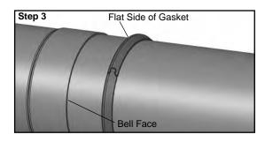
Step 3. Lubricate the gasket for best results. Install the gasket around the pipe and lock the ends together. The flat side of the gasket should be positioned against the bell face.
