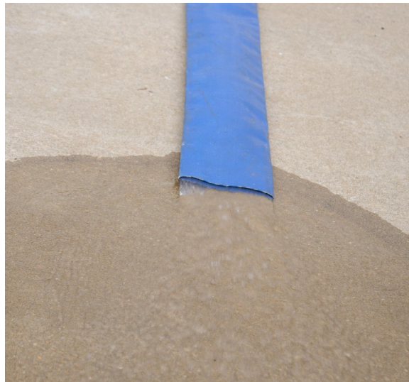
Figure 16 – Clear Water after Back-Flush
