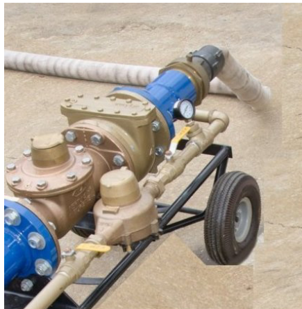
Figure 8 Hose Connection on Reference Meter
