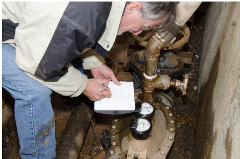
Figure 22 Meter Under Test High Side Results
