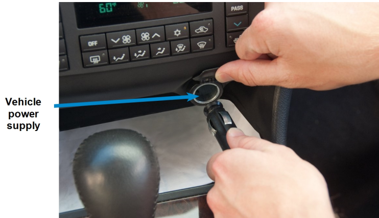
Figure 3.26 Vehicle Power Supply Cable Inserted in Car
