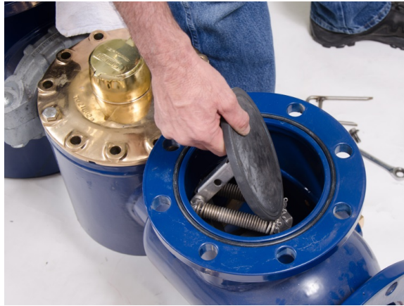
Figure 43 – Removing the Knuckle Valve
