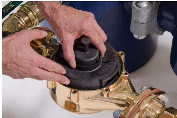
Figure 19 – Inserting the Disc Chamber
