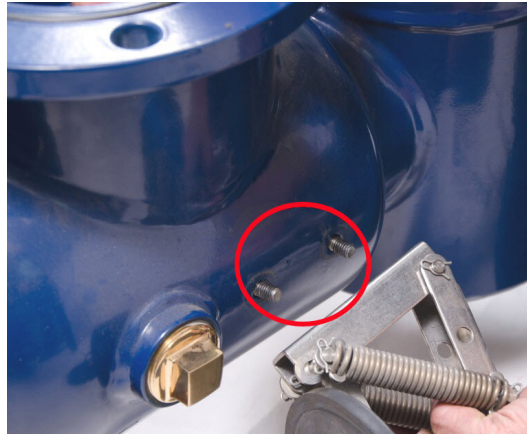
Figure 45 – Knuckle Valve Bolt Holes
