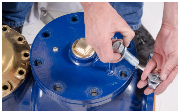
Figure 38 – Knuckle Valve Top Plate
