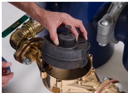
Figure 15 – T-10® Disc Chamber
