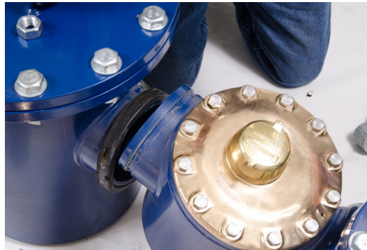
Figure 58 – Separating the Strainer
