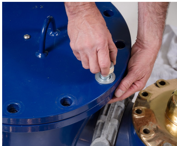
Figure 29 – Strainer Top Plate
