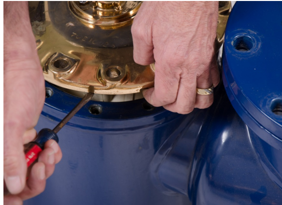
Figure 26 – Removing the HP Turbine Top Plate
