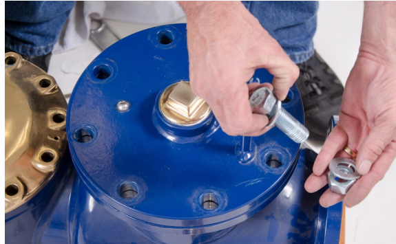
Figure 39 – Removing the Knuckle Valve Top Plate
