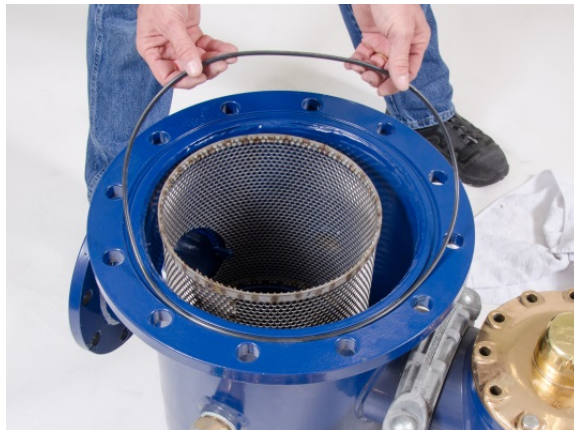
Figure 35 – Strainer Case O-Ring
