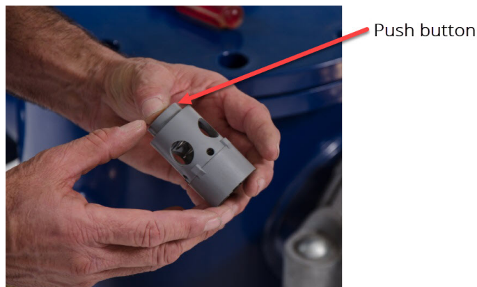
Figure 17 – Throttle Valve Push Button
