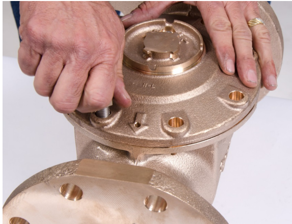
Figure 17 – Securing the Top Plate with Bolts
