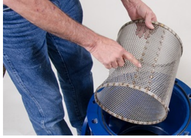
Figure 30 – Checking for Defects
