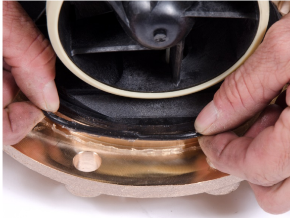
Figure 12 – Inspecting the O-Ring
