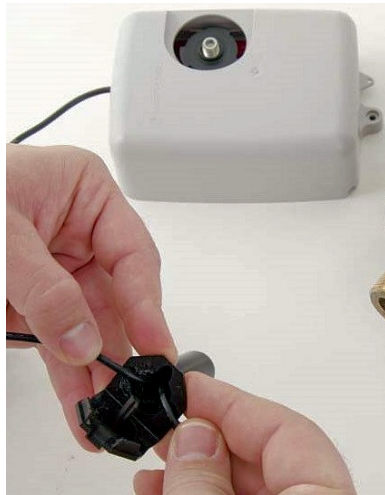
Figure 11 – Gray Wires in Slot
