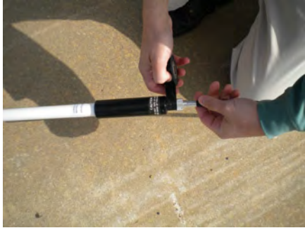
Figure 32 – Weatherizing RF Antenna
