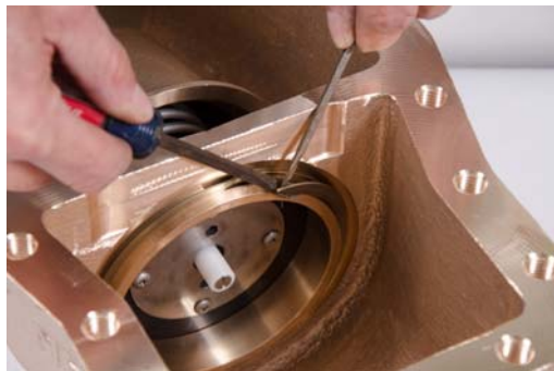
Figure 45 Dislodge the Snap Ring
