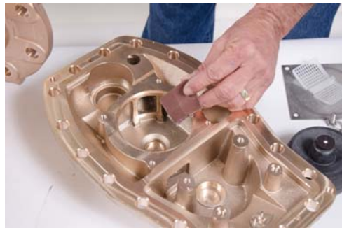
Figure 21 Cleaning Around the Chamber
