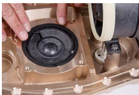
Figure 26 Replacing the Gasket
