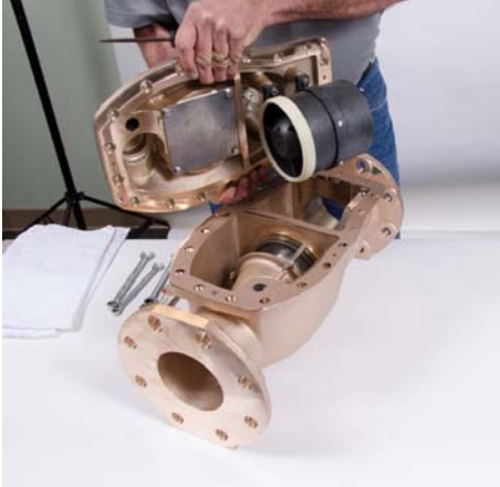
Figure 7 Unitized Measuring Element (UME)
